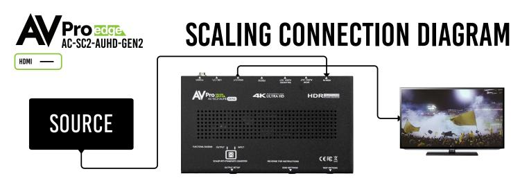
AC-SC2-AUHD-GEN2 CAN GIVE THE SINK ANY RESOLUTION FROM 480P TO 4K60 NO MATTER WHAT THE SOURCE IS OUTPUTTING
