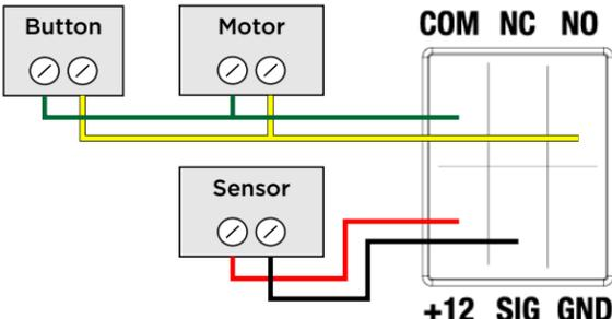
Figure 9. Connecting a dual-relay device (blinds)
