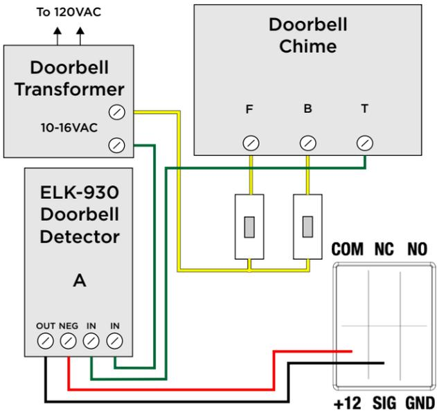
Connecting the relay ports
