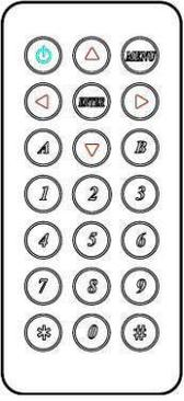
5.1 To command the matrix locally, setup the remote control IR01 ID with the same code of the Matrix (see 4.2). The default code is 4. (Power+4)
