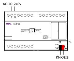
Figure 4. Wiring
