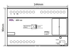
Figure 2. Dimensions - Front View
