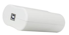
HDL-MIR01L is the Infrared Code learner. It can learn various key commands. For example, you want to control the AC, TV, DVD, Audio & Video Device, etc. IR learner can be learned into HDL BUSPRO Pro system. It has the testing mode and it do not need the extra driver.
