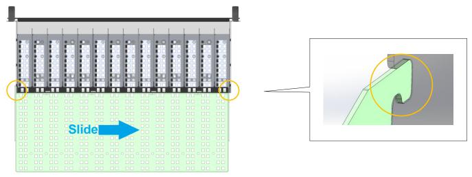
[Fig. 3] Fixing single plate
