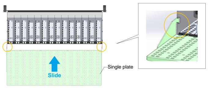
[Fig. 2] Placing single plate
