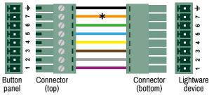
1 The cable between the button panel and the GPIO port was tested by 50 m, AWG23 cable type. For longer distance, please contact Lightware.
