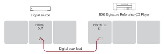
You can connect up to two digital coax inputs and two digital optical inputs to the 808 Signature Reference CD Player.
