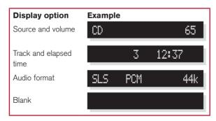
If the 808 Signature Reference CD Player has detected an authentic MQA music stream the audio format display will indicate this, and show the original sample rate as encoded in the studio.
