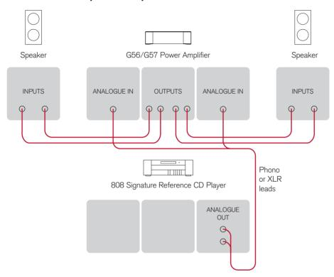
The 808 includes an integrated preamplifier, allowing you to connect it directly to a pair of analogue active loudspeakers, or to analogue passive loudspeakers via a power amplifier.
