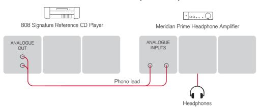
If your system uses DSP loudspeakers, you can use the analogue outputs from the 808 Signature Reference CD Player to connect to a headphone amplifier, such as the Meridian Prime Headphone Amplifier.
