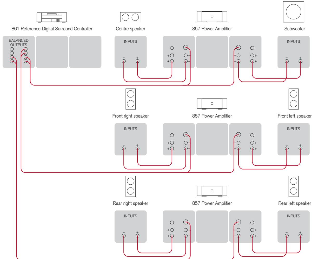
You can use three Reference Two Channel Power Amplifiers to drive the five loudspeakers and subwoofer in a surround system, using six of the balanced outputs available on the OA18 cards.
