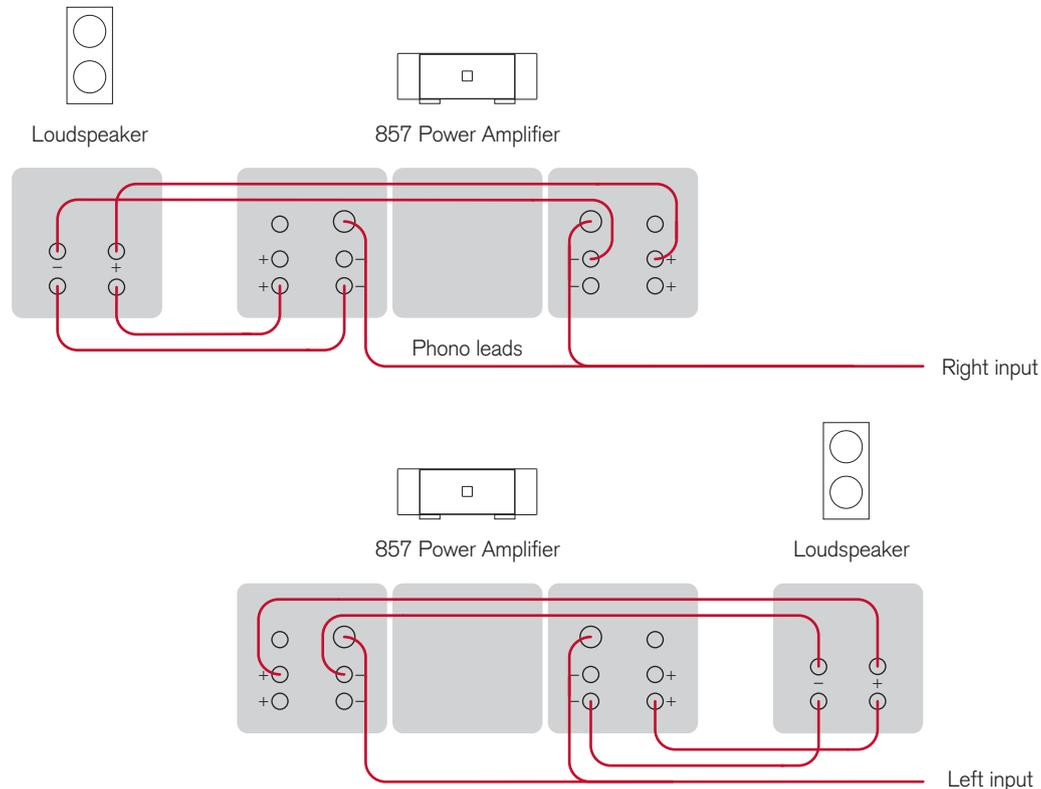
Extremely high sound quality can be achieved using two separate Reference Two Channel Power Amplifiers, one to drive each loudspeaker. The two channels in each amplifier are used to drive the LF and HF units in each loudspeaker.
