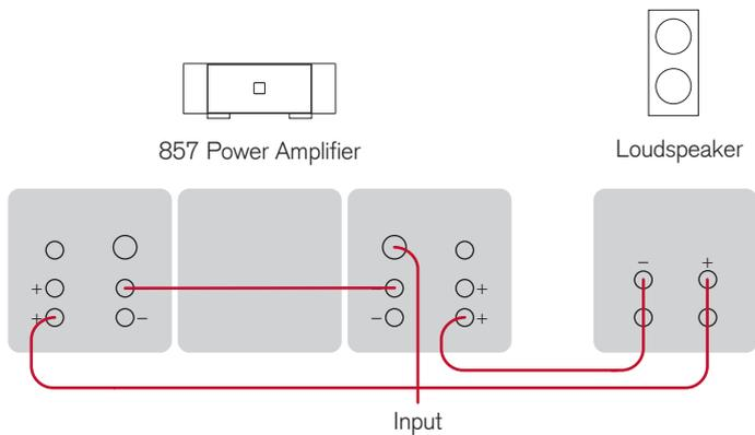
You can use the Reference Two Channel Power Amplifier as a mono power amplifier, to obtain more than twice the power output, by wiring it in bridge mode.
