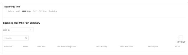
An MST instance must first be created under the *MST* tab before an MST ID can be selected. Once selected, all ports are shown, can be configured, and more detail can be viewed by selecting **Edit** for the desired interface.
