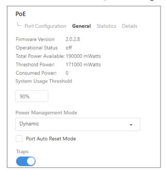
On the *General* sub-tab, edit the port's *System Threshold* or enable/disable *Power Management Mode* and *Traps*.
