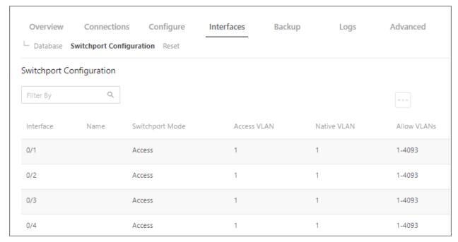
From the *Switchport Configuration* sub-tab, assign switchport settings per port. Select **Switchport Mode Access** or **Trunk**.
