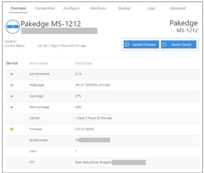
On this page, you will find information on the current firmware version, number of active ports on the switch, system-level PoE utilization, CPU and memory usage, uptime, serial number, and more.
