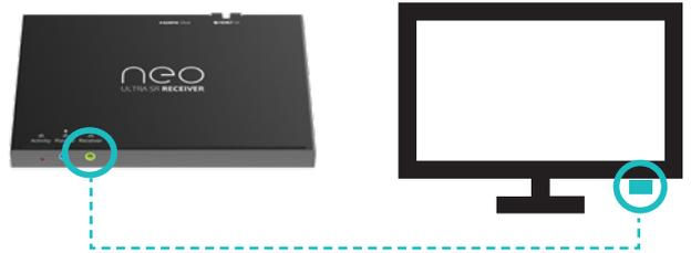
8. Finish the connection using an appropriate high speed HDMI cable from the output device and connect to the Receiver's 'HDMI Out' port.
