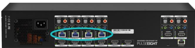
6. Complete the connection by attaching the other end of the Cat cable to a supplied neo:UltraSR Receiver's 'HDBaseT In' port. The receiver should be situated at the output end (ie. TV).
