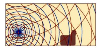
By contrast, the **Wisdom Series LS4i** speakers radiate sound as a "line source". The sound moves into the room as an expanding cylinder, rather than as an expanding sphere — as though from a vertical line suspended in space.
